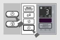
2 Set the operating time by pressing the button on the remote control or button on the unit one or more times until the desired time is displayed. The operating time can be set between 1 and 24 hours.
